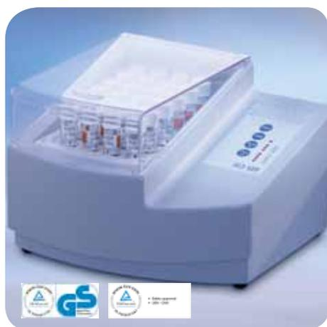
Chemical digestion of samples is required for the photometric determination of COD, TOC, total phosphate and total nitrogen.
