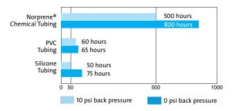
The performance of tubing in peristaltic pumping applications is affected by the conditions of use and equipment utilized, along with size and wall thickness of the tubing tested. The data above is presented for information only and should not be utilized for specification purposes.
