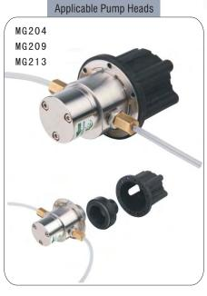
WT3000-1JA micro gear pump adopts brushless DC motor which features high efficiency and free maintenance. It can deliver flow rates from 85.7 to 2571.4 ml/min with the features of small pulse and big pressure.
