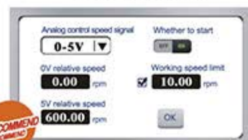
External Control Speed Setting Interface
