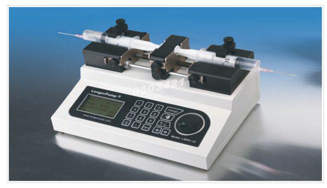
This pump is a two-syringe push-pull syringe pump. The acceptable syringes are from  $10\mu L$  to 10m L. Suitable for high accuracy and small flow rate liquid continuously transferring.
