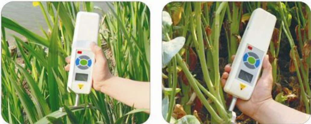
Two different fixtures for measuring the strength of different crops
